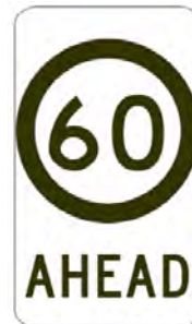
Speed Reduction Ahead Warning Sign
