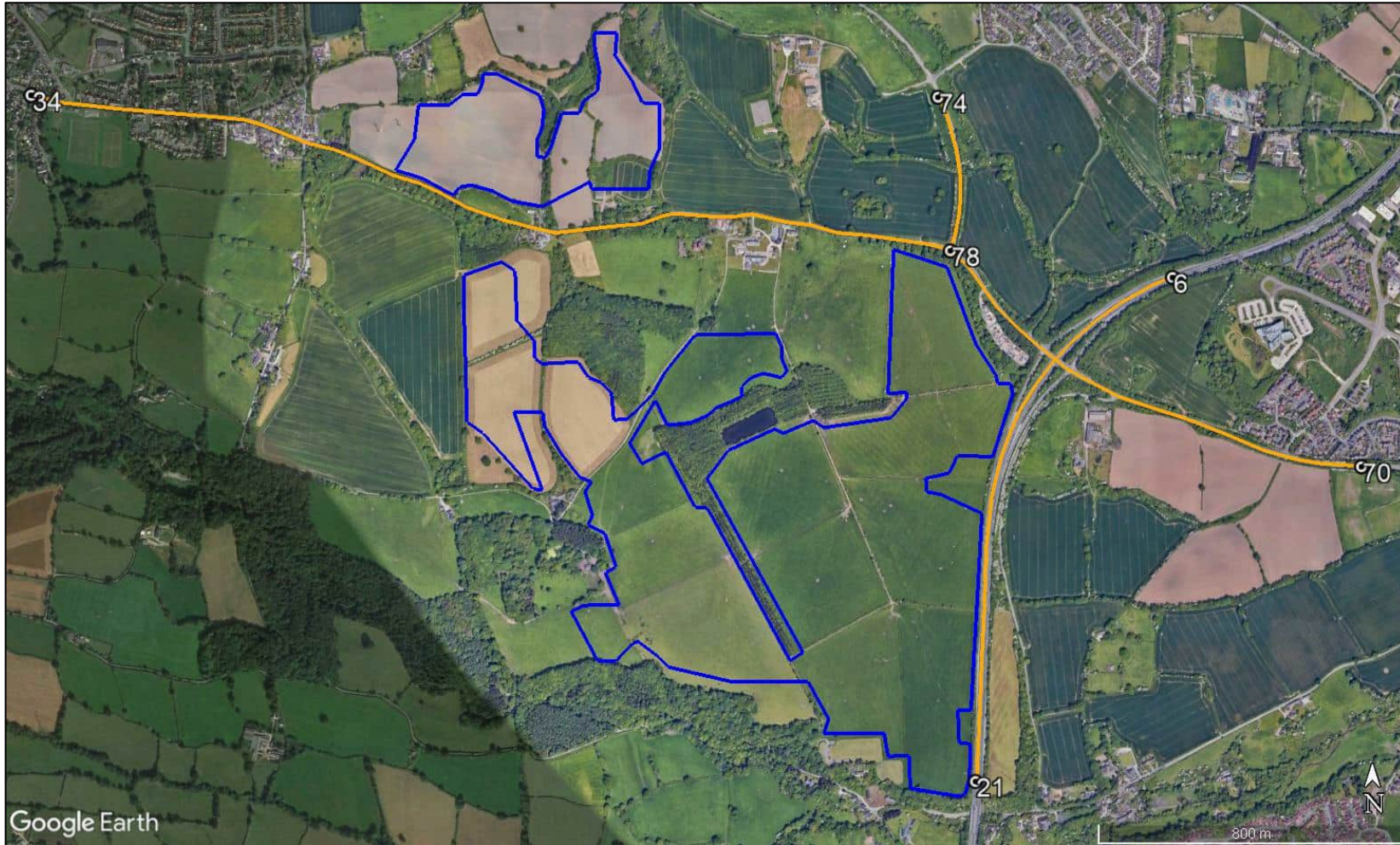
Figure 14 Sections of roads towards which solar reflections are geometrically possible (orange) – aerial image
