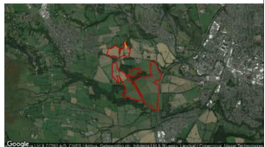
Observer Location Sun azimuth range is 275.3° - 285.2° (yellow)
