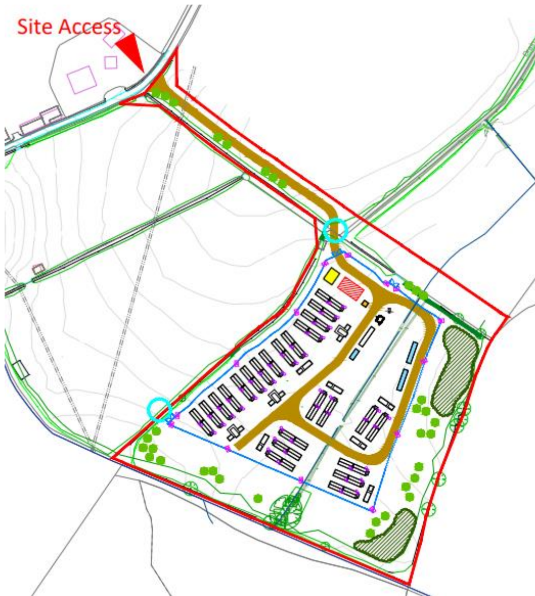
Figure 6-1 – Pentir Energy Storage Site Layout
